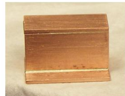
High Energy Proton Spallation of Th232 Copper Th232 target holder
