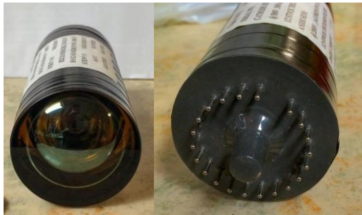
Figure C.6 Photo Multiplier Tube (Burler 8575) for Stilbene Crystal \phi 10 \text{ mm} \times 10 \text{ mm} and \phi 45 \text{ mm} \times 45 \text{ mm} .
