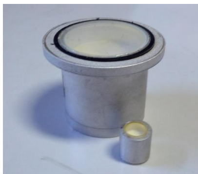
Figure 11: Stilbene Crystals \varnothing 45 \text{ mm} \times 45 \text{ mm} and \varnothing 10 \text{ mm} \times 10 \text{ mm} .
