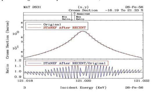
Here we see that the 7-digit output is unable to accurately define the shape of these resonances – this is IMPORTANT to understand, so let me repeat: it is PHYSICALLY IMPOSSIBLE. Rather than the smooth profile produced by the RECENT 9-digit output, the 7-digit STANEF output produces **Ziggurats** = stepped pyramids. To understand the problem we need merely compare the 9-digit RECENT output near the peak of the resonance,
