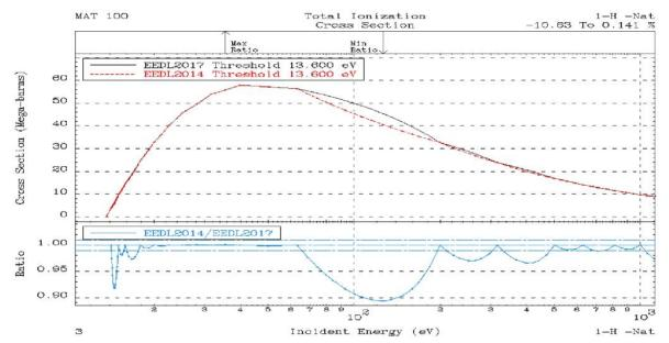
Bottom line: For EPICS2017 the documentation directs users to use lin-lin interpolation between tabulated values for both photon (EPDL) and electron (EEDL) data, and this is consistent with the interpolation laws within both ENDL and ENDF data formats which also specifies lin-lin interpolation. PLEASE: we beg users to strictly follow our recommendation and use the interpolation laws included in both ENDL and ENDF formats.
