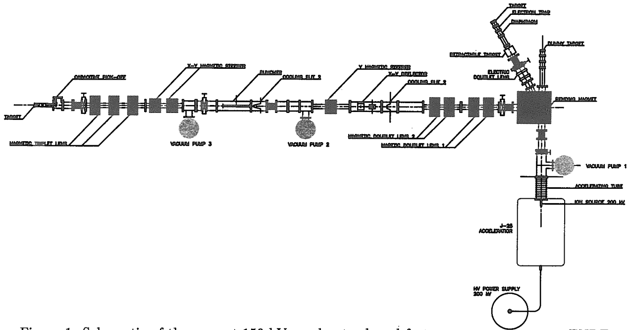
Figure 1: Schematic of the present 150-kV accelerator-based fast neutron generator at FNRF.
