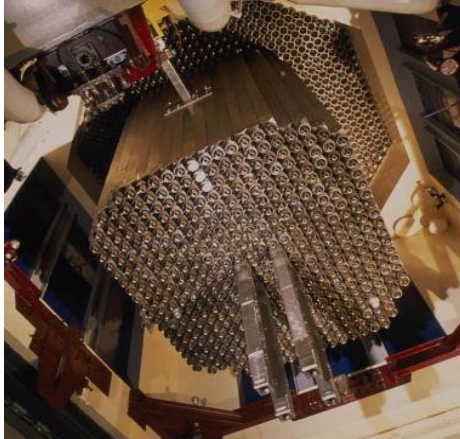
MASURCA - a fast reactor mockup of 5 kW (Cadache), presently under refurbishment
