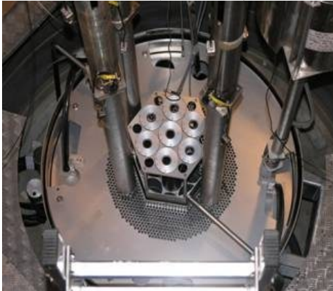
MASURCA - a fast reactor mockup of 5 kW (Cadache), presently under refurbishment
