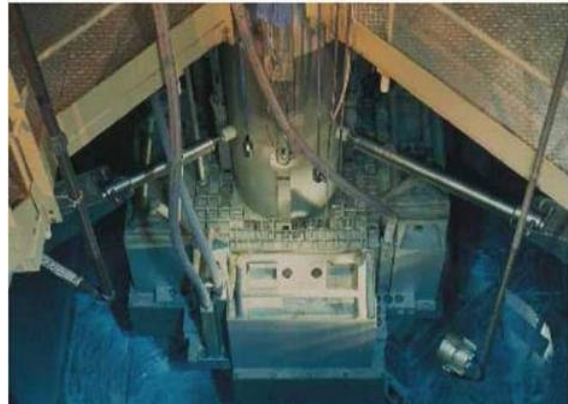
CALIBAN - ^{235}\text{U} metallic reactor (Valduc), pulse & steady state operating metallic reactor ( P < 600\text{W} )
