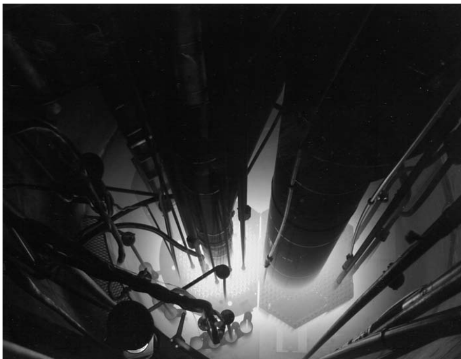
FIG. 7.1. ACRR reactor with dry central cavity (left) and external fuelled cavity (right).
